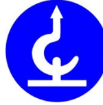
(Attachment point crane hook)
